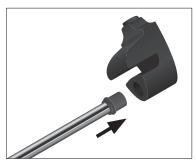
► Position the adapter on the edge of the stainless steel container.
